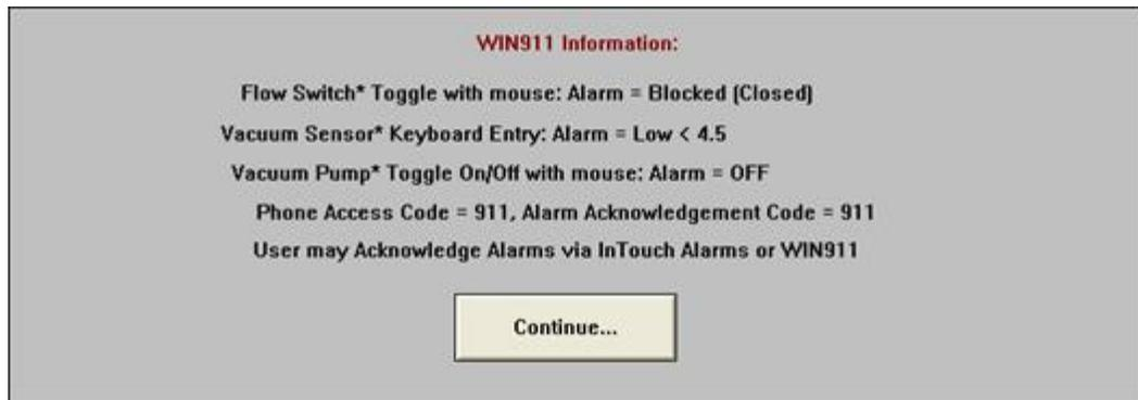
Please continue to experiment with the WIN-911 - InTouch ensemble using WIN911/411 Details to cue you in on the system alarm limits. The Pneumatic Conveyor, City Water, and Building Security operate in the same general manner, although each varies slightly to illustrate the different ways WIN-911 can be configured to process data. Modification to the InTouch Direct Connect.mdb to include pager and voice connections will give a more comprehensive demonstration of WIN-911 capabilities.
