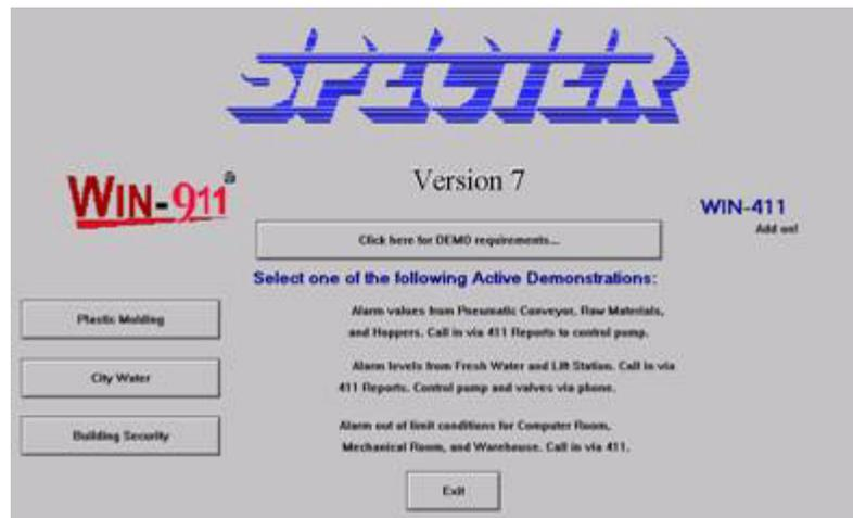
This is the main menu of the WWDEMO. From here you can toggle between the Plastic Molding, City Water, and Building Security demos. You may also review the requirements for running this demo or exit the WindowViewer program altogether. Let's start by launching the WIN-911 runtime with the InTouch Direct Connect DEMO configuration.
